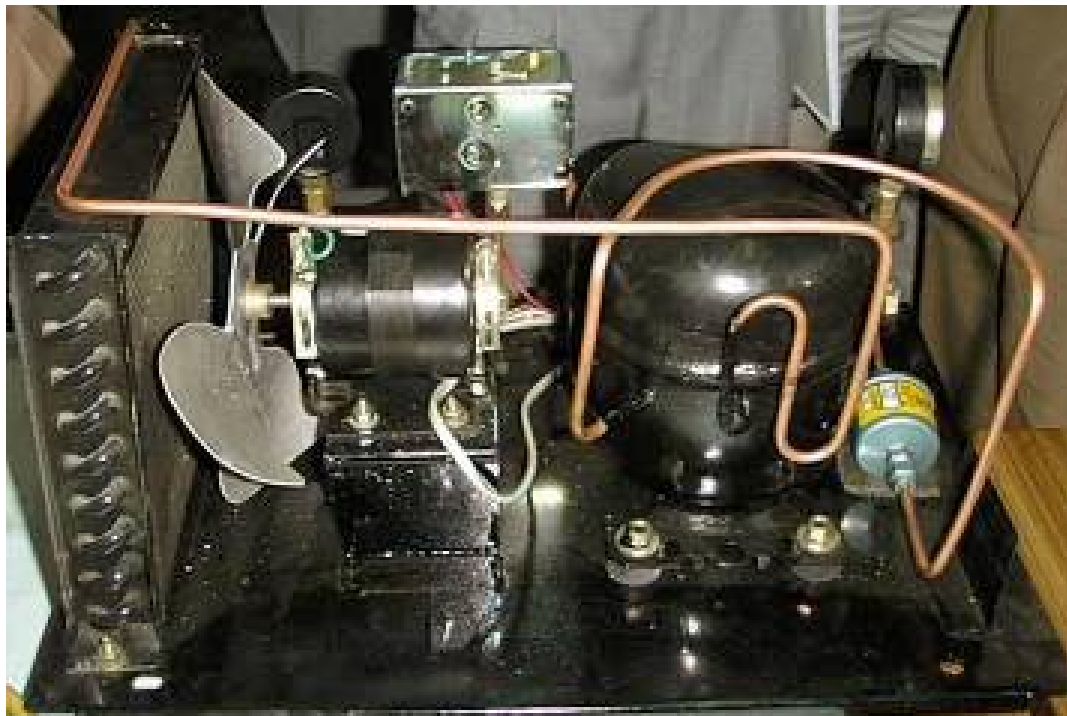
Figure A3-3 "Home made" recovery machine
