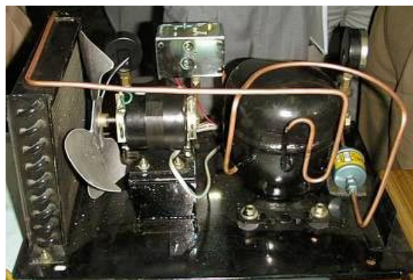
Figure 4.3, Recovery Machine made for HIDECOR workshop
