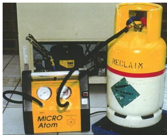
Figure 5-1, connection of recovery machine to system and cylinder
