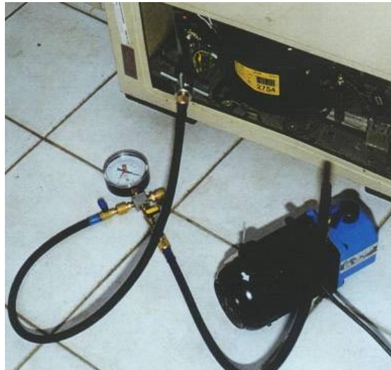
Figure 5-4, vacuum pump and gauge connected to appliance
