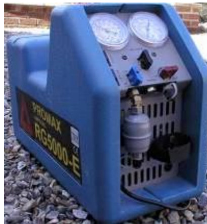
Figure 4-2, recovery machine with an oil free compressor
