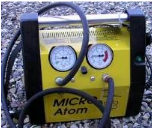
Figure 4-1, simple recovery machine of first type described above
