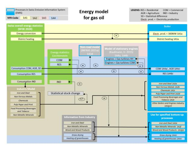
Figure 3-11 Schematic disaggregation of fuel consumption for gas oil. The Swiss overall energy statistics provides gas oil use for energy conversion and the amount thereof being used for district heating. Based on this information, gas oil use is split into the source categories 1A1ai Electricity generation and 1A1aiii Heat plants. According to the non-road model, a small amount of gas oil is consumed in source category 1A3d navigation (steam-powered vessels).
