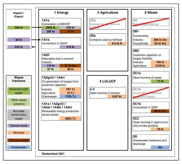
Figure 7-5 Overview on the type of treatment and amounts of waste treated in the respective sectors in Switzerland in 2021. Abbreviations: MSWIP: Municipal Solid Waste Incineration Plant, SWIP: Special Waste Incineration Plant, SSIP: Sewage Sludge Incineration Plant.
