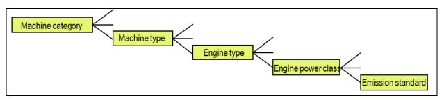
Figure 3-20 Each non-road vehicle is classified by its machine category, machine type, engine type and enginepower class and emission standard (FOEN 2015j, INFRAS 2015a). The emission modelling is based on activity data and emission factors by means of the following equation, which holds on the most disaggregated level of engine power class (Figure 3-20):
