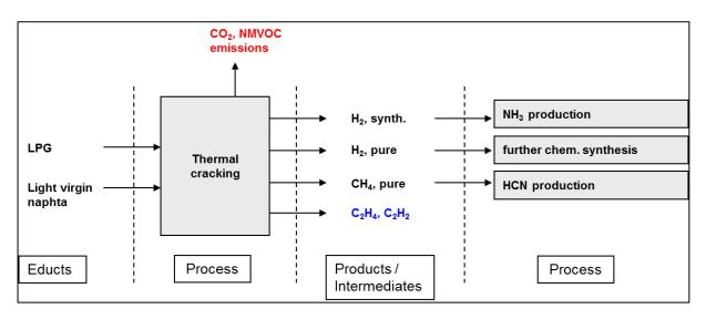
Figure 4-6 Process flow chart for the production of ethylene ( $C_2H_4$ ) and acetylene ( $C_2H_2$ ) by thermal cracking of liquefied petroleum gas (LPG) and light virgin naphtha. The intermediate product  $H_2$ , synth. is used as educt in the ammonia production in the same plant.
